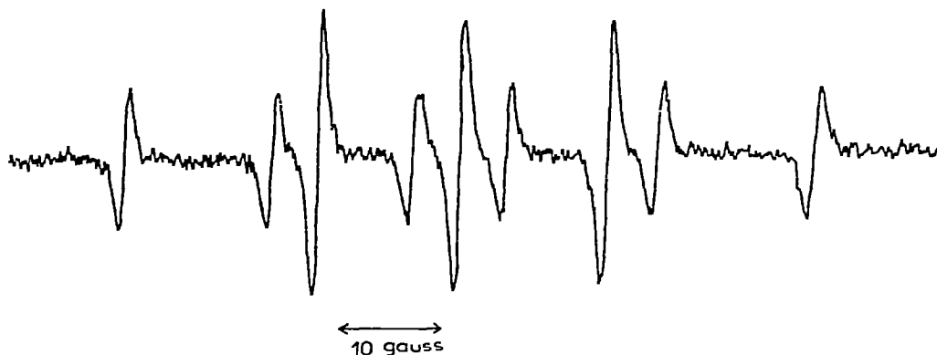
Fig. 1. ESR spectrum of the hydrogen atom spin adduct to DMPO from the photolysis of methylpyridine-cobaloxime in benzene containing DMPO (0.05 mol). Modulation amplitude 1.0 G, microwave power 20 mW.
